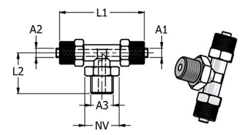
Hose diameter A1 = 10/8Hose diameter A1 = -Hose diameter A2 = 10/8L1 = 45L2 = 27.5NV = 16Thread A3 = G 1/4"
